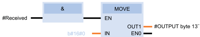
Figure 4: Output bit 0 of byte 13 write to megacontrol If input bit = 1 then output is 0
