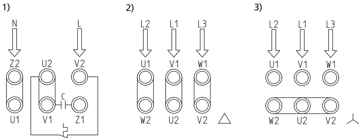
Figure 6: Wiring diagram, depending on selected motor
