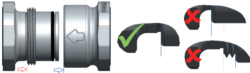
Fig. 18: Verifying the alignment
